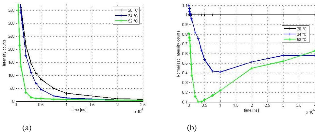
**Figure 2:** (a) Intensity dependency of acetone at  $P = 15,000$  Pa for varying temperature at a 310 nm wavelength excitation, (b) data normalized with the intensity values at 20 °C
